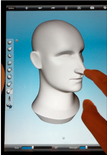
figure 2. Mesh deformation in 123D Sculpt. A drag gesture is used to grab and pull the nose mesh. There are limited parameters for each tool. The geometry of the mesh is not visible to the user, nor is the axial system of the 3D environment.
